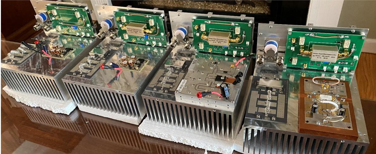
Amplifiers for 50, 144, 222 and 432 MHz with key components mounted
